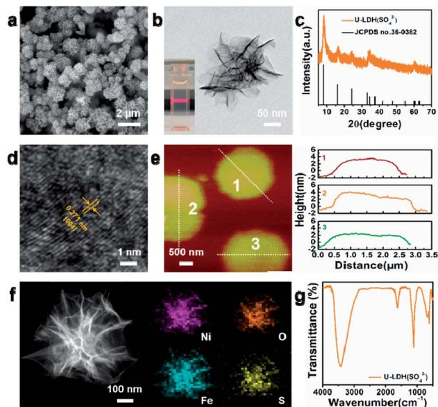
Fig. 1 (a) SEM image, (b) TEM image, (c) PXRD patterns, (d) HRTEM image, (e) AFM image and height profiles, (f) HAADF-STEM image and EDX elemental mappings, (g) FT-IR spectrum of the U-LDH(SO<sub>4</sub><sup>2-</sup>). The inset in (b) shows the Tyndall light scattering of the U-LDH(SO<sub>4</sub><sup>2-</sup>) in aqueous solution.
