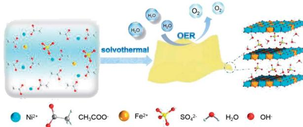
Scheme 1 Synthetic procedure for U-LDH(SO<sub>4</sub><sup>2-</sup>) nanosheets and its application in oxygen evolution reaction (OER).
