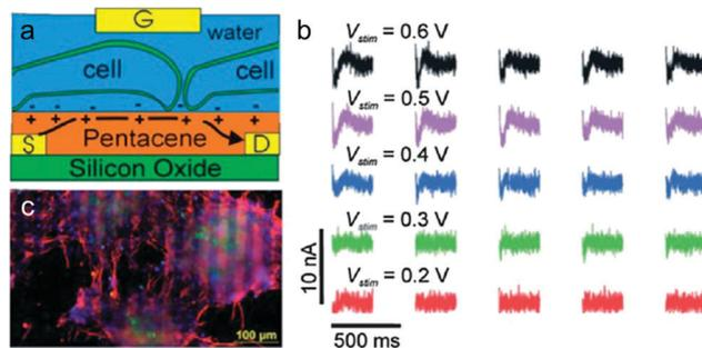
**Fig. 15** Water-gated organic field effect transistors (WGOFET) neuronal transducer. (a) Schematic model of the device and interactions with adhering cells. (b) Drain current time traces recorded from a differentiated network after stimulation with various intensities. (c) Fluorescent microscopy image which indicates the formation of a functional neuronal network derived from murine stem cells on the transistor surface.<sup>262</sup>
