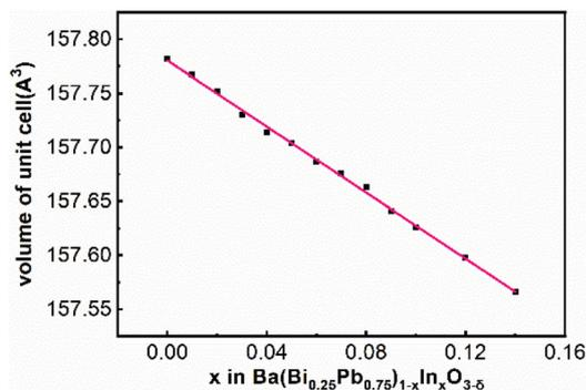
Fig. 7 Volume of the unit cell of Ba(Bi<sub>0.25</sub>Pb<sub>0.75</sub>)<sub>1-x</sub>In<sub>x</sub>O<sub>3-δ</sub> at room temperature.
