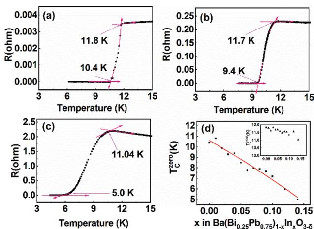
Fig. 10 Temperature-dependent resistance of In1 (a), In5 (b) and In13 (c), and composition-dependent  $T_c^{\text{zero}}$  of  $\text{Ba}(\text{Bi}_{0.25}\text{Pb}_{0.75})_{1-x}\text{In}_x\text{O}_{3-\delta}$  (d).
