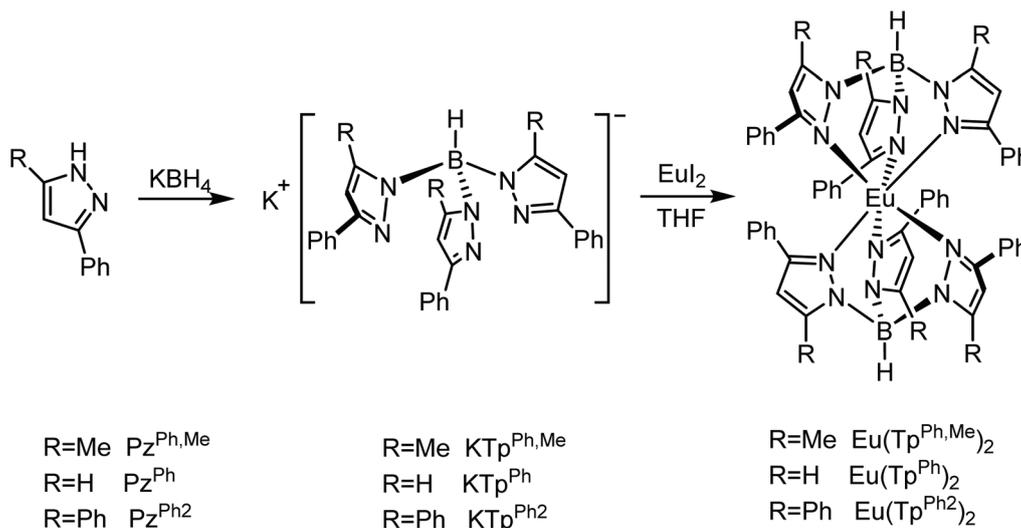
Scheme 1 Synthetic routes of  $\text{Eu}(\text{Tp}^{\text{Ph,Me}})_2$ ,  $\text{Eu}(\text{Tp}^{\text{Ph}})_2$  and  $\text{Eu}(\text{Tp}^{\text{Ph}_2})_2$ .
