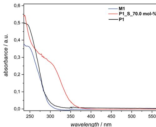
Fig. 5 UV-Vis spectra of **M1**, **P1** and **P1\_S\_70.0 mol%**. Sample concentrations were  $1.23 \times 10^{-5} \text{ mmol mL}^{-1}$  (for **M1**) and  $6.25 \times 10^{-2} \text{ mg mL}^{-1}$  (for **P1** and **P1\_S\_70.0 mol%**.) in THF. Solvent cut-off wavelengths  $\lambda_0$ : 215 ( $\lambda_{\text{max}}$ : 220 nm in THF). For details, refer to the main text and the ESI.†
