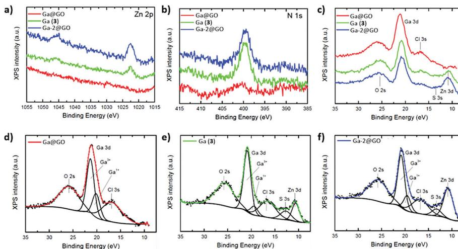
**Fig. 6** XPS spectra of core levels (a) Zn 2p, (b) N 1s, (c) Ga 3d. (d) Ga 3d energy region for the Ga@GO sample with a fit of a  $\text{Ga}^{3+}$ , 3 Ga–O singlet,  $\text{Ga}^{1+}$ , and Ga–Cl, (e) and (f) same scenario than (d) but for the Ga (3) and Ga-2@GO samples.
