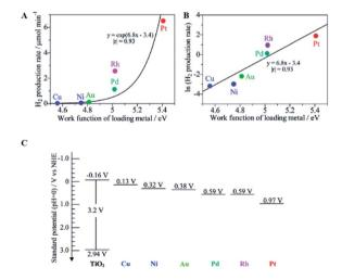
Fig. 3 Relationship between the hydrogen production rate over the M(0.1)/TiO $_2$  samples and the work function of the corresponding bulk metal (A), the logarithmic plot (B), and the standard potentials for the band edge positions of titanium oxide and the Fermi level of each loading metal (C). Reprinted with permission from ref. 62. Copyright 2012 American Chemical Society.
