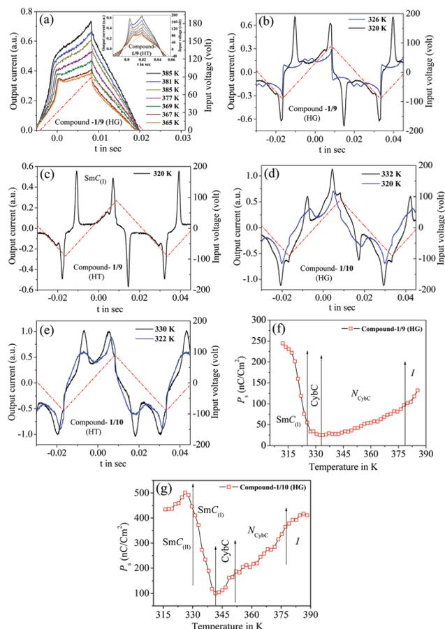
**Fig. 7** Switching current response curves of compounds **1/9** and **1/10** for a triangular wave voltage (red dashed line) at different temperatures; (a–c) compound **1/9** in the HG cell, (d) compound **1/10** in the HG cell, (e) compound **1/10** in the HT cell, (f and g) temperature-dependent polarization value for compounds **1/9** and **1/10**, respectively.
