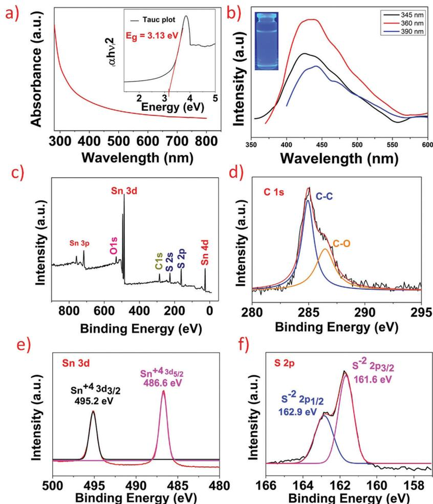
Fig. 3 (a) UV-Visible absorption spectra of  $\text{SnS}_2$  QDs; the inset is the Tauc plot showing a bandgap of  $\sim 3.13$  eV. (b) Photoluminescence spectra of  $\text{SnS}_2$  QDs at different excitation from 345 nm to 390 nm. (c) XPS survey spectra of  $\text{SnS}_2$  QDs. (d) High resolution spectra of C 1s. (e) High resolution spectra of Sn 3d. (f) High resolution spectra of S 2p.
