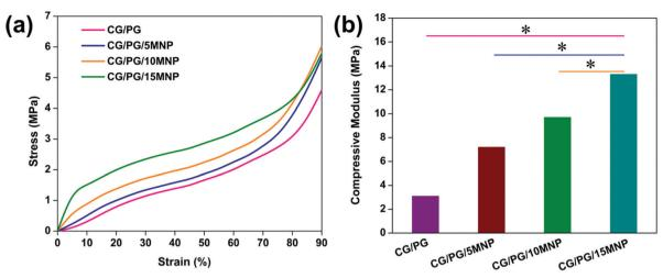
Fig. 5 (a) Stress-strain curve and (b) compressive modulus of CG/PG, CG/PG/5MNP, CG/PG/10MNP and CG/PG/15MNP composite scaffolds.
