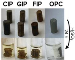
Fig. 5 Appearance of terpenoid–sulfur composite (A) or of ordinary portland cement (OPC) and composite-infused portland cement (B) compressional test cylinders before and after submersion in 0.5 M  $\rm H_2SO_4$  for 24 h.
