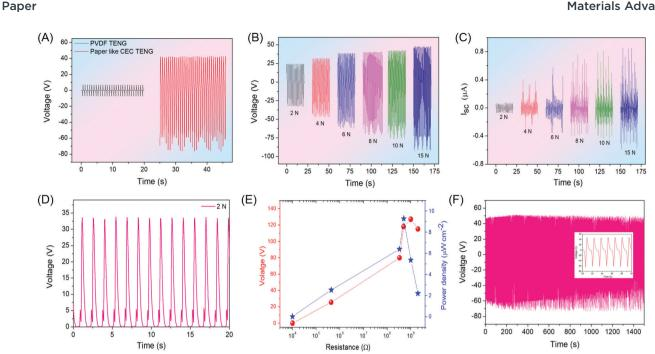
Fig. 5 (A) Relative output voltage of the PVDF and P-CEC-based TENG, (B and C) output voltage and current of the P-CEC TENG as a function of applied compressive force, respectively, (D) rectified voltage of the P-CEC TENG at a constant applied compressive force of 2 N, (E) output voltage and maximum peak power of the P-CEC TENG as a function of load resistance, and (F) endurance test of the P-CEC TENG over 1500 s at a constant applied force.
