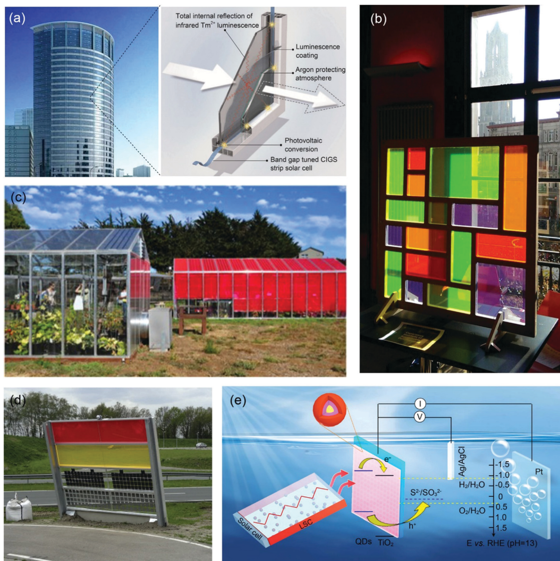
Fig. 15 (a) Schematic of a PV window consisting of a semi-transparent, colorless LSC. (b) Photograph of the Electric Mondrian prototype. (c) Photograph of the LSC greenhouse. (d) Photograph of the noise barrier prototype. (e) Schematic diagram of the CdSe/CdS/CdS QD sensitized photoanode coupled with an LSC based on CdSe/CdS QDs. (a) Reproduced with permission from ref. 28. Copyright 2015 Elsevier. (b) Reproduced with permission from ref. 149. Copyright 2017 Wiley-VCH. (c) Reproduced with permission from ref. 150. Copyright 2016 AIP publishing. (d) Reproduced with permission from ref. 151. Copyright 2017 Elsevier. (e) Reproduced with permission from ref. 153. Copyright 2019 The Royal Society of Chemistry.
