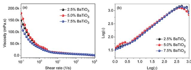
Fig. 3 (a) Shear rate dependence of viscosity and (b) logarithmic plot of shear stress of the slurries with various BaTiO<sub>3</sub> loadings.
