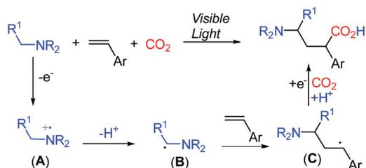
Scheme 2 Photocatalytic preparation of  $\gamma$ -amino acids from  $\text{CO}_2$ .
