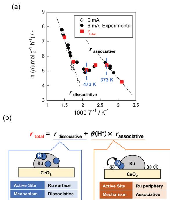
Fig. 13 Temperature dependence of  $\text{NH}_3$  synthesis rate ( $r$ ) without the electric field ((a), open plot), in the electric field ((a), black closed plot) and overall reaction rate ((a), red closed plot), calculated based on the concept shown in (b).
