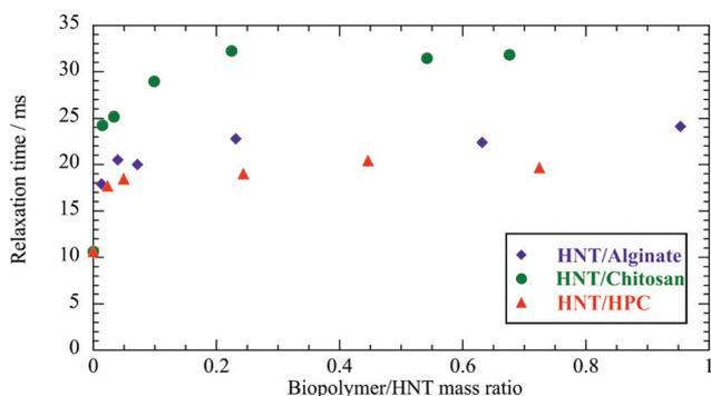
Fig. 5 Relaxation time determined by the fitting of the EBR data as a function of the biopolymer/HNT mass ratio at a HNT concentration of  $0.15 \text{ g dm}^{-3}$  (SANS and FCS experiments were done at 0.1).
