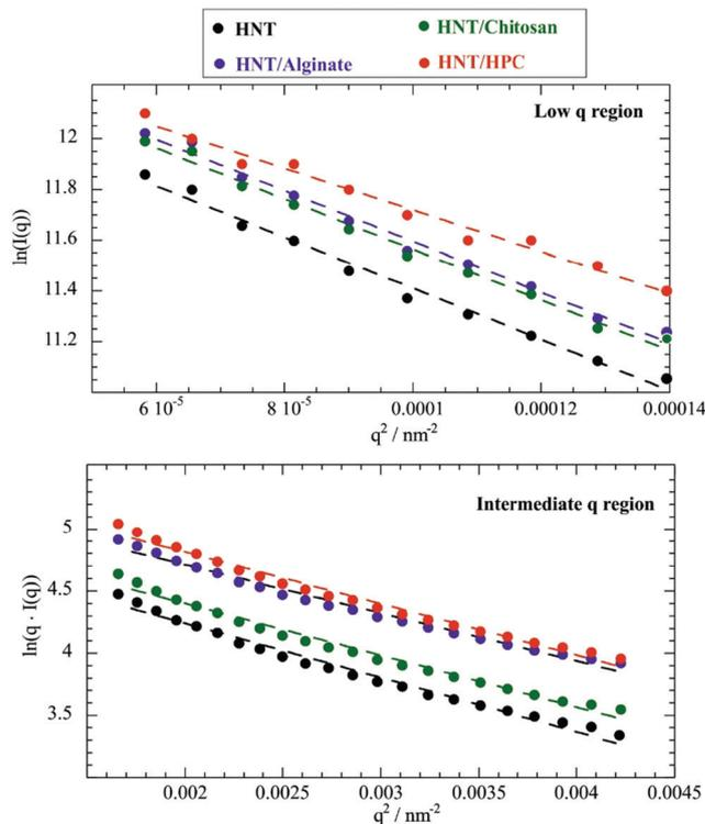
Fig. 2 Guinier plots for HNT/chitosan, HNT/alginate, HNT/HPC and HNT dispersions in  $\text{D}_2\text{O}$  within the low ( $0.007 \text{ nm}^{-1} \leq q \leq 0.009 \text{ nm}^{-1}$ ) and the intermediate ( $0.015 \text{ nm}^{-1} \leq q \leq 0.02 \text{ nm}^{-1}$ ) regions. The low  $q$  Guinier plot is  $\ln(I(q))$  vs.  $q^2$  (top), while the intermediate  $q$  Guinier plot is  $\ln(q \cdot I(q))$  vs.  $q^2$  (bottom). Dashed lines represent the fitting according to eqn (1) and (3).
