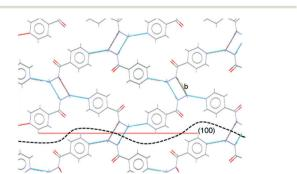
Fig. 12 Overlay of the (100) plane (red line) with the underlying bulk IZN crystal structure in Mercury. "b" highlights discrete NH···N intermolecular hydrogen bonding interactions formed between adjacent hydrazine moieties. The black dashed line represents a hypothetical real surface termination for the (100) face, assuming only cleavage of intermolecular interactions.
