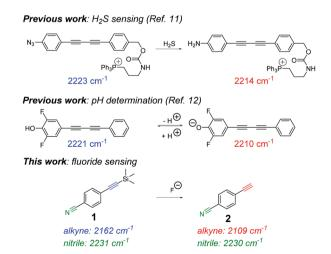
Fig. 1 Previous reports of sensing and quantification using alkyne-tag Raman imaging. (i) A previous example of an irreversible sensor for hydrogen sulfide (H<sub>2</sub>S) detection<sup>11</sup> and (ii) a reversible sensor for quantifying intracellular pH.<sup>12</sup> This work reports an extremely low molecular weight Raman sensor (1) for ratiometric detection of fluoride ions.
