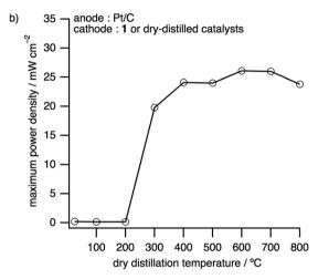
Fig. 5 Maximum power densities of  $H_2-O_2$  fuel cells depending on the dry distillation temperature. At the dry distillation temperature of 25 °C, 1 is used as it is as a fuel cell catalyst. (a) Anode: 1 or DDCs. Cathode: Pt/C. (b) Anode: Pt/C. Cathode: 1 or DDCs.
