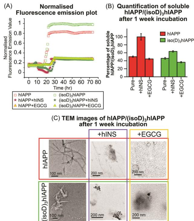
Fig. 3 (A) Normalised fluorescence emission plot of 50  $\mu$ M hIAPP and (isoD)<sub>3</sub>hIAPP solutions with equimolar hINS and EGCG. (B) MS quantification of 10  $\mu$ M hIAPP and (isoD)<sub>3</sub>hIAPP with equimolar inhibitors after 1 week incubation and (C) TEM images of fibrils found in solutions after 1 week incubation at 37  $^{\circ}$ C.
