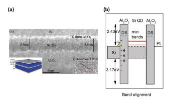
Fig. 2 TEM cross-section and sketch of an ESC based on silicon QDs (a). The QDs are sandwiched between thin layers of  $Al_2O_3$  to form a double barrier resonant tunnelling structure. The sketch in (b) shows the involved energy levels with the discrete levels of Si QDs within the barrier. Copyright 2017, published by Wiley-VCH.
