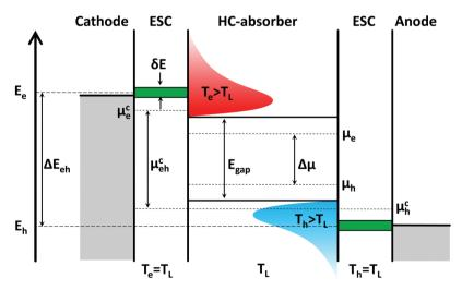
Fig. 1 The proposed scheme of a hot carrier solar cell working under non-equilibrium conditions involves an absorber layer in which charge carriers cool only slowly towards the lattice temperature  $T_L$ . The extraction of such hot carriers occurs through energetically narrow selective contacts (ESCs, green) to isentropically cool down the carriers. This process allows to generate a larger splitting of the quasi-Fermi levels or a higher chemical potential  $\mu_c^{
