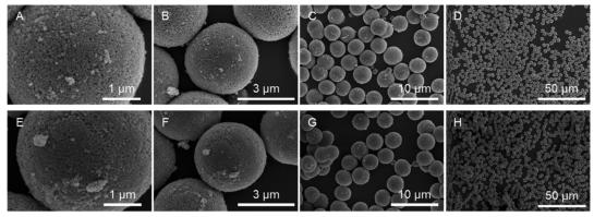
Fig. 2 SEM images of (A-D): bare CaCO<sub>3</sub> particles and (E-H): polymer-modified CaCO<sub>3</sub>-PMAcO particles.
