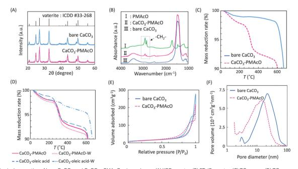
Fig. 3 Physical properties of bare CaCO<sub>3</sub> and CaCO<sub>3</sub> - PMAcO microspheres: (A) XRD spectra, (B) FT-IR spectra, (C) TG curves, (D) TG curves of CaCO<sub>3</sub> -PMAcO and CaCO<sub>3</sub>-oleic acid before and after washing; "-W" indicates samples after washing, (E) N<sub>2</sub> adsorption-desorption isotherms, and (F) poresize distributions
