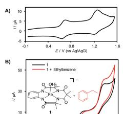
Fig. 1 (A) CV of  $[(TAML)Fe^{III}(OH_2)]Na$  (1) in  $CH_3CN$  (0.1 M LiClO<sub>4</sub>). (B) CVs of 0.5 mM 1 in the absence (black) and presence (red) of 20 mM ethylbenzene in 1:1 CH<sub>3</sub>CN: H<sub>2</sub>O and K<sub>2</sub>HPO<sub>4</sub> (0.1 M). The increase in the current of the (TAML)Fe redox feature at 1.25 V (vs. Ag/AgCl) is attributed to catalytic ethylbenzene oxidation by a high-valent Fe-oxo species generated at this potential. Scan rate = 50 mV s<sup>-1</sup>.
