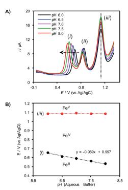
Fig. 2 (A) Differential pulse voltammograms of 0.5 mM 1 in 1:1  $\rm CH_3CN$ : buffer (0.1 M phosphate). (B) Pourbaix diagram derived from the peak potentials of redox features (i) and (iii) in (A).
