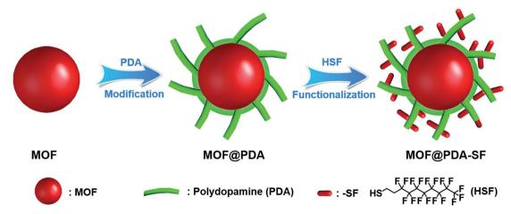
Fig. 1 The modification process used to prepare hydrophobic MOF@PDA-SF composites.
