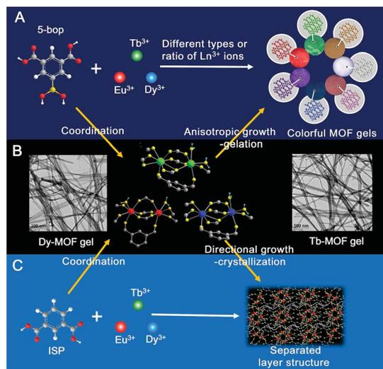
Fig. 1 (A) The selection of different types and ratios of  $\text{Ln}^{3+}$  ions for the formation of MOF gels with different colors. (B) The formation of Tb- and Dy-MOF gels because of their different coordination environments compared to that of  $\text{Eu}^{3+}$ . (C) Separated layer structure revealed from single crystal results for the formation of nanoribbons, which entangle together to form MOF gels.
