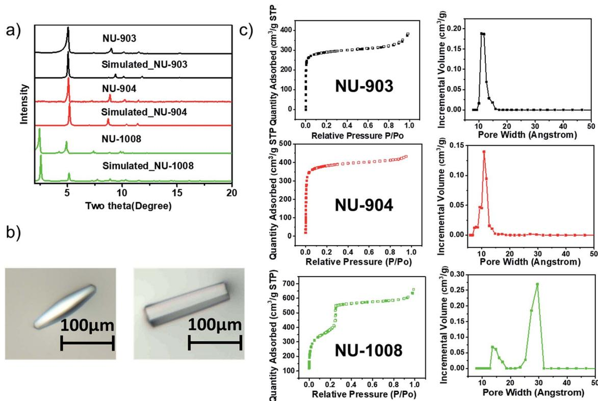
Fig. 3 Characterization of the three MOFs. (a) PXRD patterns; (b) optical images of the single crystals of NU-904 (left) and NU-1008 (right), the scale bars in the images are 100  $\mu\text{m}$ ; (c)  $\text{N}_2$  sorption isotherms and DFT pore size distribution of NU-903, NU-904 and NU-1008.
