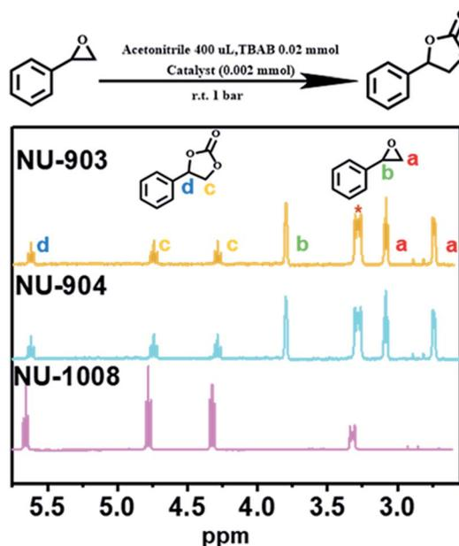
Fig. 5 Proton NMR spectra of CO<sub>2</sub> fixation into styrene oxide catalyzed by NU-903, NU-904 and NU-1008 (1 bar, room temperature, 24 h; CDCl<sub>3</sub> as deuterium solvent, 500 MHz). The peak with asterisk refers to the tetrabutylammonium bromide.
