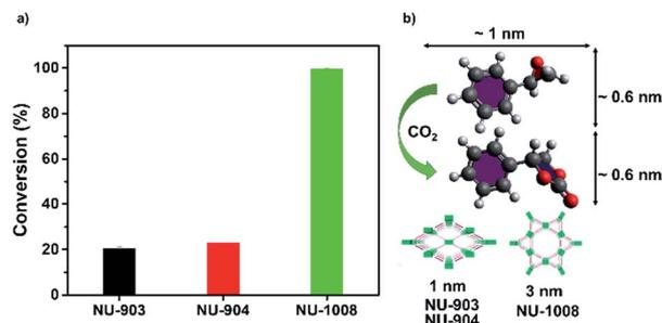
Fig. 6 CO<sub>2</sub> fixation conversion on NU-903, NU-904 and NU-1008. (a) Catalytic capacities; (b) size of substrate, product and pore size of NU-903, NU-904 and NU-1008.
