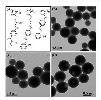
Fig. 6 (A) The molecular structures of P1, P2, and P3 that have similar pendant structures and molecular weight to PHAzoMA<sub>59</sub>, for further confirming the formation mechanism and demonstrating the extensibility of this design strategy to prepare nanobowls; (B), (C) and (D) TEM images of HCMs from P1 and P2, and nanobowls from P3, respectively
