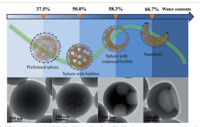
Fig. 5 Evolution of nanobowls from PHAzoMA<sub>226</sub>. With the addition of water, PHAzoMA<sub>226</sub> forms preformed spheres, spheres with bubbles, spheres with coalesced bubbles and nanobowls at different water contents. The TEM images show the corresponding nanostructures at the various water contents from left to right.
