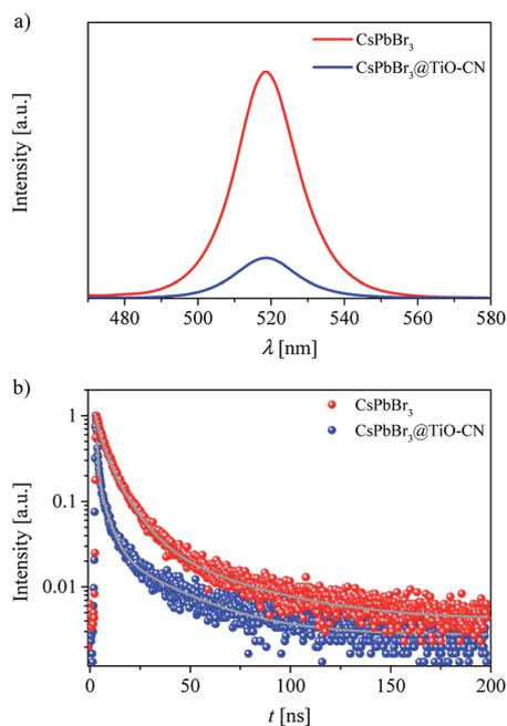
Fig. 4 (a) Photoluminescence spectra of  $CsPbBr_3$  and  $CsPbBr_3@TiO-CN$ . (b) Time-resolved photoluminescence decays of  $CsPbBr_3$  and  $CsPbBr_3@TiO-CN$ . The gray curves are the fitting lines based on a multi-exponential function.
