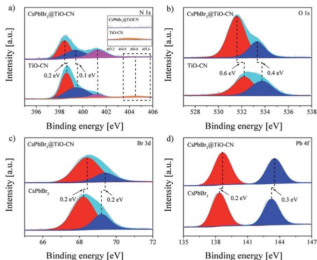
Fig. 2 High-resolution XPS spectra of CsPbBr<sub>3</sub>, TiO-CN and CsPbBr<sub>3</sub>@TiO-CN: (a) N 1s, (b) O 1s, (c) Br 3d and (d) Pb 4f.
