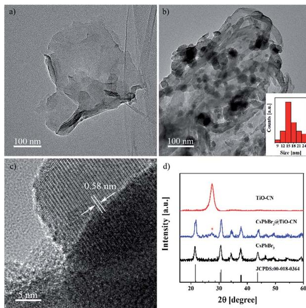
Fig. 1 TEM images of TiO-CN (a) without and (b) with CsPbBr<sub>3</sub> nanocrystal loading. The black dots in panel b are the CsPbBr<sub>3</sub> nanocrystals, and the particle size distribution of CsPbBr<sub>3</sub> is given in the inset in panel b. (c) HRTEM image with the lattice spacing of monoclinic CsPbBr<sub>3</sub> on TiO-CN. (d) XRD patterns of TiO-CN, CsPbBr<sub>3</sub> and CsPbBr<sub>3</sub>@TiO-CN.
