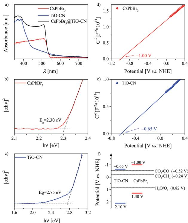
Fig. 3 (a) UV/Vis diffuse reflectance spectra of CsPbBr<sub>3</sub>, TiO-CN and CsPbBr<sub>3</sub>@TiO-CN. Tauc plots of (b) CsPbBr<sub>3</sub> and (c) TiO-CN. Mott-Schottky plots of (d) CsPbBr<sub>3</sub> and (e) TiO-CN. (f) Schematic illustration of the band structures of CsPbBr<sub>3</sub> and TiO-CN derived from the results of flat-band potential and UV/Vis diffuse reflectance spectroscopy measurements.
