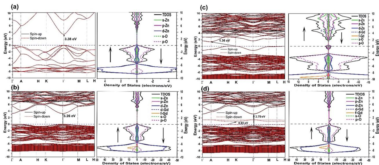
Fig. 10 The electronic band structures, TDOS and PDOS of (a) pristine ZnO, (b) Gd-doped ZnO, (c)  $\text{Gd}_{\text{Zn}}-\text{V}_{\text{O}}$  complex and (d)  $\text{Gd}_{\text{Zn}}-\text{V}_{\text{Zn}}$  complex.
