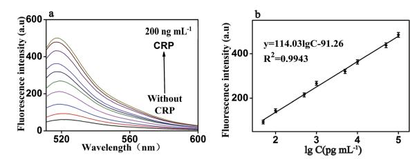
Fig. 6 (a) Fluorescence emission spectra of the biosensor in the presence of CRP with different concentrations: from bottom to top: 0 to 200 ng  $mL^{-1}$  (b) The fluorescence intensity as a function of CRP concentration. It shows the strong correlation between fluorescence intensity and CRP concentration, under both experimental conditions: RNA, 50 nM; P1, 20 nM; RNase H, 8 U; GO, 20  $\mu$ g mL<sup>-1</sup> and the emission wavelength of 519 nm. Error bars: SD, n=3.
