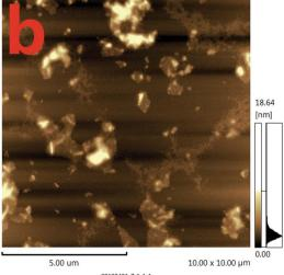
Fig. 3 The atomic force microscopy (AFM) images of different mixtures. (a) The AFM image of GO dripping directly on the surface of mica; (b) the AFM image of the mixtures of GO with microRNAs on the surface of mica. The concentrations of GO and microRNAs were 20 μg mL<sup>-1</sup> and 20 nM, respectively. The volume of GO and microRNAs were both of 6 μL.
