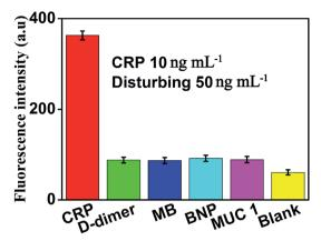
Fig. 7 Fluorescence intensity (at the emission wavelength of 519 nm) of the sensor in the presence of CRP (10 ng mL $^{-1}$ ), D-dimer (50 ng mL $^{-1}$ ), MB (50 ng mL $^{-1}$ ), BNP (50 ng mL $^{-1}$ ), MUC 1 (50 ng mL $^{-1}$ ) and blank, respectively. Error bars: SD, n=3.
