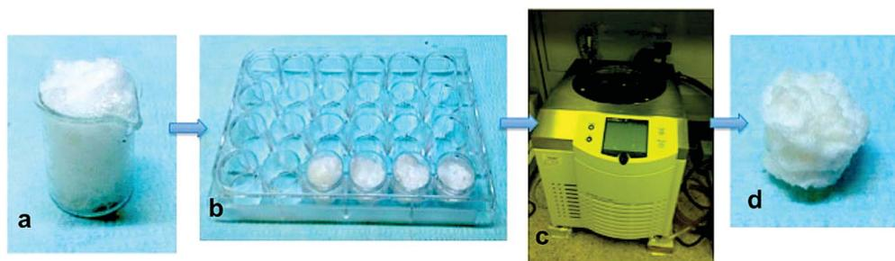
Fig. 1 Schematic representation of the fabrication method: the polymeric foam was obtained from the gas foaming process during which the generated carbon dioxide is incorporated into the polymer (a). The PVA foam was poured in a mold (b), frozen at  $-20\text{ °C}$  for 6 h, freeze-dried for a 24 h, (c) and then the scaffolds were extracted from the mold (d).
