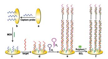
Fig. 14  $\,$  A schematic representation of the preparation of the hybridization chain reaction-based ECL DNA sensor. <sup>108</sup> Reprinted with permission from ref. 108. Copyright 2012 American Chemical Society
