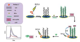
**Fig. 2** A schematic representation of the modification of the GCE and the detection of ATP. <sup>31</sup> Reprinted with permission from ref. 31. Copyright 2016 American Chemical Society.
