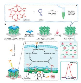
Fig. 11 Schematic illustration of (A) the fabrication procedure of the ABEI-Ag@PAni-PA conducting hydrogel, (B) the preparation of the ECL biosensor for cell assay, and (C) the  $H_2O_2$  production path triggered by the PMA and ECL reaction mechanism. 103 Reprinted with permission from ref. 103. Copyright 2018 American Chemical Society.
