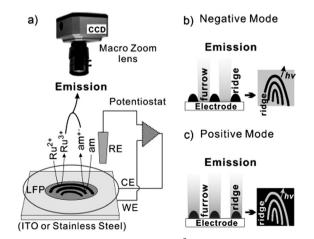
Fig. 15 (a) The ECL imaging system:  $Ru^{2+}$  and am represent the ECL generating luminophore and the amine co reactant, respectively. (b and c) The imaging strategy for visualizing LPFs in the negative (b) and positive (c) mode. 109 Reprinted with permission from ref. 109. Copyright 2012 Wiley-VCH Verlag GmbH & Co. KGaA, Weinheim.
