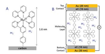
Fig. 18 (A) Structure of the  $Ru(bpy)_3^{2+}$  molecular layer deposited on a carbon substrate. (B) A schematic illustration of the Cr<sub>4</sub>/Au<sub>30</sub>/eC<sub>10</sub>/Ru(bpy)<sub>3</sub>P/ eC<sub>10</sub>/Au<sub>20</sub> molecular junction. Reprinted with permission from ref. 119. Copyright 2017 American Chemical Society.
