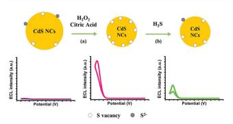
Fig. 5 (a) Schematic representation of activation of CdS QDs by  $H_2O_2$  and citric acid (b) its application in H<sub>2</sub>S detection based on the quenching effect of ECL emissions caused by adsorption of H<sub>2</sub>S on the surface S vacancies.<sup>62</sup> Reprinted with permission from ref. 62. Copyright 2014 American Chemical Society.
