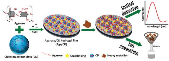
Fig. 6 Fabrication of an agarose/carbon-dot/hydrogel film optical sensor for heavy metal ion detection. <sup>17</sup>
