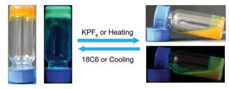
Fig. 3 Optical and fluorescent photographs of the reversible gel-sol transition of TPE-based fluorescent polymer hydrogels.<sup>29</sup> (left) Upon cooling or 18C<sub>6</sub> addition, TPE-hydrogel in its solidified gel state with bluegreen fluorescent emission image side by side; (right) Upon KPF<sub>6</sub> addition or heating, the hydrogel turns liquid, and lost its fluorescence intensity as seen in the stacked images of the hydrogel in normal light and UV illumination.
