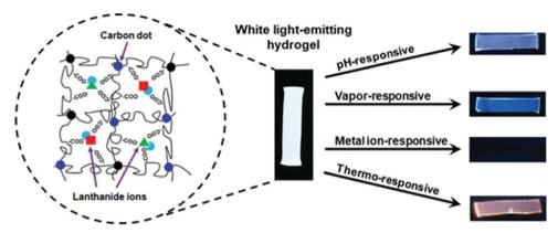
Fig. 9 A white light emitting hydrogel sensor incorporating lanthanide ions and carbon dots and color-responsive to environmental cues including pH, chemical vapors, ions, and temperature. 48
