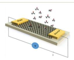
Fig. 5 A schematic design of the flat or patterned MLG-based sensors for E/I/A-containing cancer marker detection. Graphene is placed on a flexible PVC substrate of 25  $\mu$ m thickness. A two-point measurement concept was used for the *in situ* electrical characterization of CM-induced graphene electrodes and its selectivity analysis.
