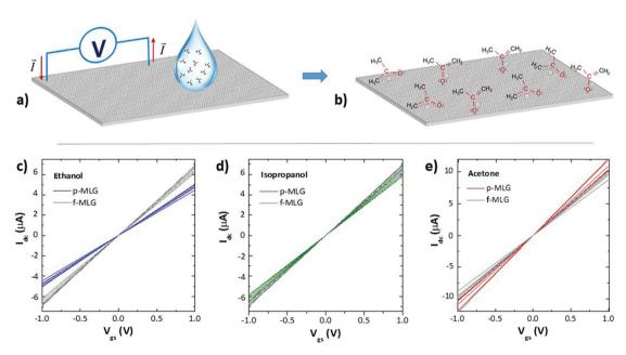
Fig. 3 The schematic representation of the two-point measurement concept (a) for the in situ electrical characterization of VOC-induced graphene electrodes (c, d); electron-induced reorientation of acetone while applying  $\pm 1$  V (b). The  $I_{dc}$  versus  $V_{gs}$  curves of the flat and patterned graphene electrodes influenced with exposure to  $1.4-3.3 \times 10^5$  ppm of VOC solutions: ethanol (c), isopropanol (d) and acetone (e).
