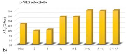
Fig. 6 Selectivity analysis for cancer marker detection by monitoring the sheet resistance value for the three types of organics in various combinations with f-MLG (a) and p-MLG-based (b) electrodes: single solutions of ethanol (E), isopropanol (I), acetone (A); double solutions -E+I+A, and A+I; and the triple solution -E+I+A.
