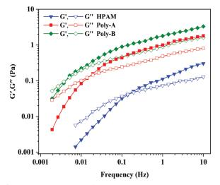
Fig. 9 Viscoelastic behavior of copolymers.
