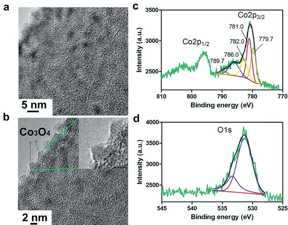
Fig. 2 TEM (a) and HRTEM (b) images of Co100@nCNFs. The inset shows the crystalline spinel structure of Co<sub>3</sub>O<sub>4</sub> nanoparticles. Deconvoluted XPS spectra of Co2p (c) and O1s (d) for Co100@nCNFs.
