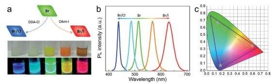
Fig. 8 (a) Schematic of anion exchange with DDACl and OAml for blue and red spectra, and the corresponding solution samples after anion exchange (blue to red from left to right). (b) The PL spectra of typical samples from blue to red. (c) Solid line area is CIE coordinates of NCs after anion exchange, and the dashed area is the standard NTSC TV color.
