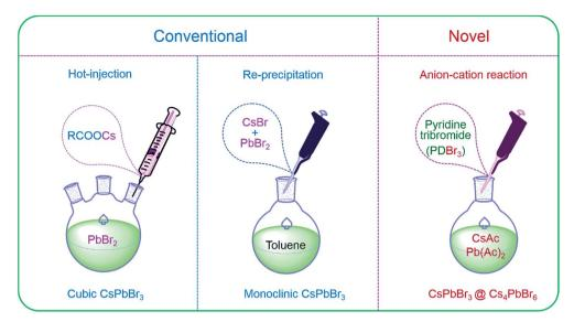
Fig. 2 Schematic of the hot-injection, re-precipitation and anion-cation reactions for cubic CsPbBr<sub>3</sub>, monoclinic CsPbBr<sub>3</sub> and CsPbBr<sub>3</sub>@-Cs<sub>4</sub>PbBr<sub>6</sub> NCs.
