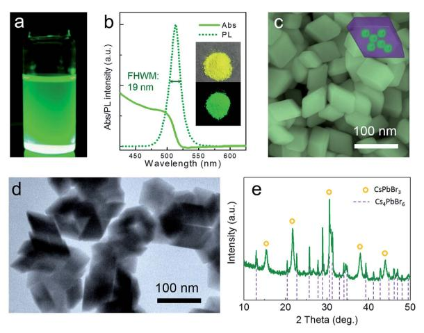
Fig. 3 Typical CsPbBr<sub>3</sub>@Cs<sub>4</sub>PbBr<sub>6</sub> sample: (a) toluene dispersion under UV light. (b) PL and absorption spectrum. Inset: photographs of powder sample under day light and UV light, respectively. (c) SEM image of typical CsPbBr3@Cs4PbBr6. Inset: schematics of the microstructure. (d) TEM image of the typical CsPbBr3@Cs4PbBr6. (e) XRD pattern of the typical CsPbBr3@Cs4PbBr6.
