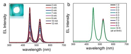
Fig. 9 (a) EL spectra of the CsPbBr $_3$ @Cs $_4$ PbBr $_6$  NC powder-based backlit LED under different currents; inset is the photograph of the backlit LED. (b) EL spectra of the CsPbBr $_3$ @Cs $_4$ PbBr $_6$ -based backlit LED lighted for 10 days under ambient conditions.
