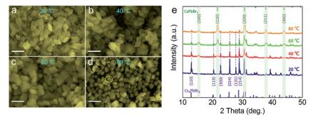
Fig. 5 SEM images of products prepared at different temperatures: (a) 20 °C, (b) 40 °C, (c) 60 °C and (d) 80 °C. (e) The corresponding XRD patterns of products prepared at different temperatures.
