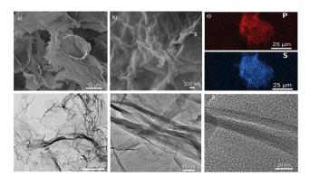
Fig. 2 Microscopic analyses of DG<sub>4</sub>-GO. (a and b) SEM of DG<sub>4</sub>-GO. (c) EDX mapping of phosphorus (up) and sulfur (bottom). (d) TEM and (e and f) HRTEM of DG4-GO.
