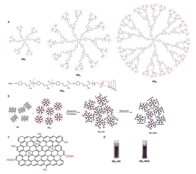
(a) Chemical structures of dendrimers  $DG_n$ . (b) Illustration of the exfoliation of layered graphitic oxide materials by ammonium-terminated phosphorus dendrimers and their subsequent reduction. (c) Structures of GO. (d) Digital photos of  $DG_1$ -GO and  $DG_1$ -RGO dispersion in aqueous solution.
