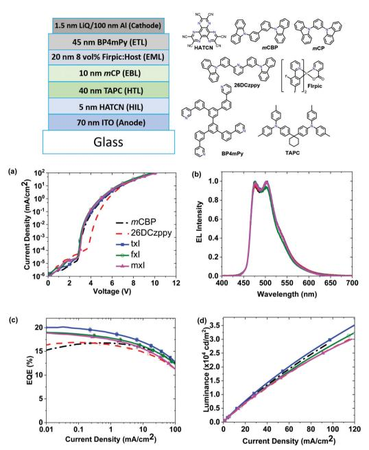
Fig. 5 OLED device characteristics of phenanthro[9,10-d]imidazole and reference hosts. (top) Device architecture and chemical formula of materials. (a) J-V curves. (b) EL spectra. (c) Efficiency versus current curves. (d) Luminance versus current curves.
