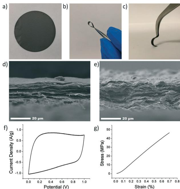
**Fig. 4** Digital images of (a) an rGO electrode and (b and c) an rGO/ANF composite electrode (no CNTs). Cross-sectional SEM images of (d) an rGO/ANF electrode without CNTs (95/5 wt% rGO/ANFs) and (e) with 20 wt% CNTs (76/4/20 wt% rGO/ANFs/CNTs). (f) A representative cyclic voltammogram and (g) a typical stress–strain curve for an rGO/ANF/CNT composite electrode (90.25 wt% rGO, 4.75 wt% ANFs, 5 wt% CNTs).
