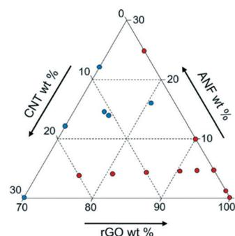
**Fig. 2** Ternary diagram describing the design space for rGO/ANF/CNT supercapacitor electrodes. Original experimental data are plotted with red circles while predicted compositions which were then validated experimentally are plotted with blue circles.
