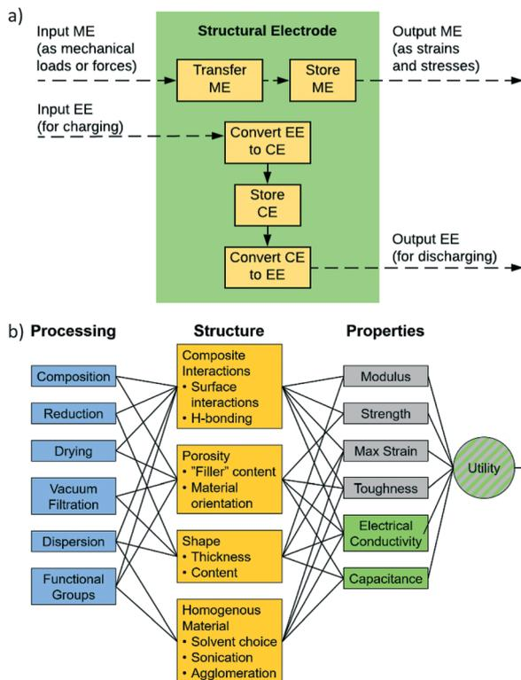
**Fig. 1** (a) Component level functional diagram of a typical structural electrode where ME is mechanical energy, EE is electrical energy, and CE is chemical energy. In this diagram, the structural electrode can discharge electrical energy while also safely handling mechanical loads. (b) Material level system chart of the interactions between the process, structure, and properties within a composite electrode consisting of ANFs, graphene, and CNTs.
