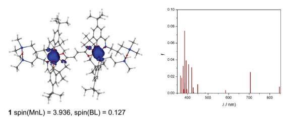
Fig. 11 Visualisation of spin density, including spin density populations on the Mn - tetradentate Schiff base moiety MnL and on the bridging ligand BL (left) and calculated TD-DFT transitions (right) of the neutral 1 (nonet) species. The values of spin densities are in a.u. The isovalue was set to ±0.005 a.u.
