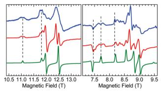
Fig. 8 Fragments of HFEPR spectra of 1 at 406.4 GHz and 10 K (left) and 2 at 203.2 GHz and 10 K (right). Blue: Experimental. Red: Calculated using spin Hamiltonian 2 (dimer model, eqn (2)). Green: Calculated using spin Hamiltonian 1 (monomer model, eqn (1)). The indicated splittings appear also in other regions of the spectra, and at different frequencies.
