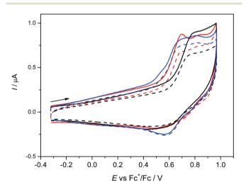
Fig. 3 Cyclic voltammograms of 0.15 mM 1 (red traces), 2 (black traces) and 3 (blue traces) in nBu<sub>4</sub>NPF<sub>6</sub>/CH<sub>2</sub>Cl<sub>2</sub> (GC-disc working electrode, scan rate 100 mV s<sup>-1</sup>, solid line – the first voltammetric scan, dashed line - the second scan).
