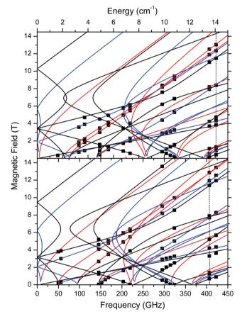
**Fig. 9** Field vs. frequency/energy map of turning points in complexes **1** (top) and **2** (bottom) at 10-15 K. Squares are experimental points; curves were simulated using spin Hamiltonian parameters as in Table 2. Red curves: turning points with magnetic field  $B_0$  parallel to the x-axis of the ZFS tensor; blue:  $B_0 \mid\mid y$ ; black:  $B_0 \mid\mid z$ . The two dashed vertical lines indicate the frequencies at which spectra shown in Fig. 6 were recorded.
