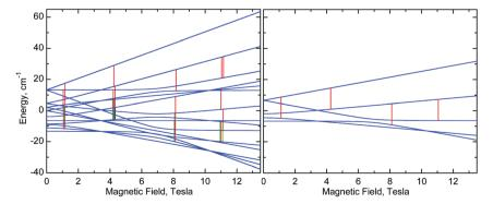
Fig. 10 Right: Energy levels of a monomer, calculated at the "z" orientation, using eqn (1) with parameters of 1 (Table 2). Left: Energy levels of a dimer, calculated using eqn (2) with the same single-ion g, D and E parameters of 1 and with J = -0.025 cm<sup>-1</sup>. The vertical lines represent EPR transitions expected at  $\nu = 406.4$  GHz. Only transitions with substantial probability are drawn. Colours are used to distinguish very close transitions. See also Fig. S8, ESI.†
