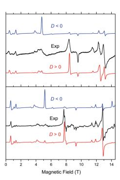
**Fig. 6** Low-temperature HFEPR spectra of **1** at 422.4 GHz and 15 K (top) and **2** and 406.4 GHz and 10 K (bottom, both represented as black traces) accompanied by simulations using S = 2 spin Hamiltonian parameters as in Table 2. Blue traces: simulations using negative D; red traces: positive D.
