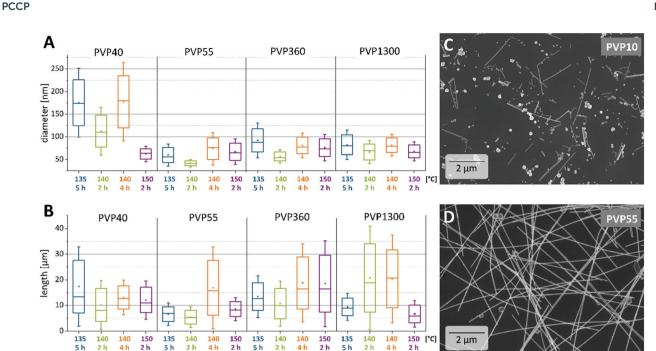
Fig. 1 (A) Diameters and (B) lengths of the AgNWs synthesized at different reaction temperatures, times and  $M_{\rm w}$  of PVP. The corresponding colours in different frames reflect the same reaction temperature and time. (C) SEM images of the AgNWs synthesized at 140 °C for 2 h with (C) PVP10 or (D) PVP55.
