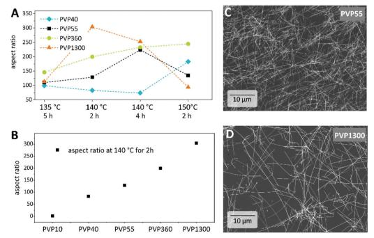
Fig. 2 Aspect ratios of the synthesized AgNWs with various  $M_{\rm w}$ s of PVP obtained at (A) different reaction temperatures and times and (B) 140 °C for 2 h. SEM images of the AgNWs synthesized at 140 °C for 2 h in the presence of (C) PVP55 or (D) PVP1300.
