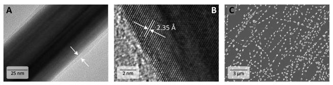
Fig. 3 (A) TEM image of a AgNW clearly shows a PVP shell, (B) HR-TEM image of a AgNW showing a lattice distance of 2.35 Å corresponding to the (100)-facet, and (C) SEM image of a destroyed AgNW network after gradual annealing until 250 °C.
