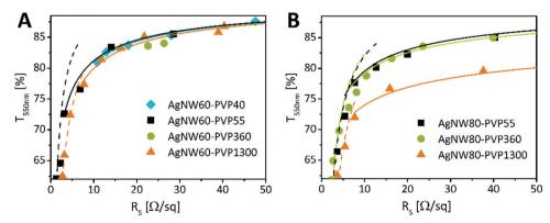
Fig. 4 Sheet resistance versus transmittance at 550 nm of AgNWs varying in the PVP-shell with (A) 60 nm and (B) 80 nm diameter. The dashed lines correspond to bulk behavior, and the continuous line corresponds to percolative behavior. Fitted with a model presented by De et al.<sup>39</sup>
