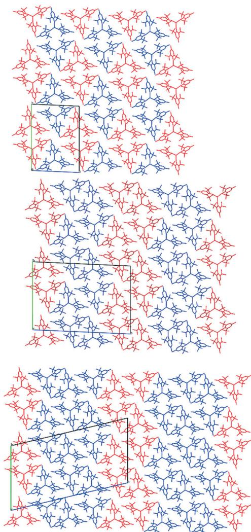
**Fig. 4** Crystal structures of **1** at 140 K (top), 120 K (middle) and 100 K (bottom), viewed along the *a*-axis with the unit cell highlighted. Planar conformations are shown in blue and pyramidal in red.
