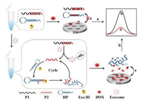
Scheme 1 Principle of the aptamer recognition-trigged label-free homogeneous electrochemical strategy for ultrasensitive detection of cancerderived exosomes
