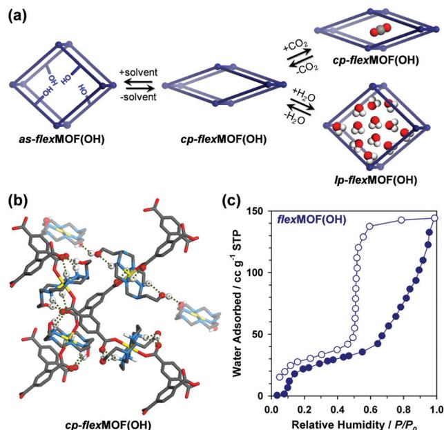
Fig. 5 (a) Schematic illustration of the phase transitions of *flexMOF(OH)* upon guest removal/reintroduction and adsorption/desorption of  $\text{CO}_2$  and  $\text{H}_2\text{O}$  molecules. (b) Hydrogen bonds of *cp-flexMOF(OH)* as represented by dotted lines, and (c) its water vapour isotherm at 298 K. Filled and empty circles represent adsorption and desorption curves, respectively.
