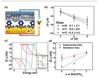
Fig. 3 (a) A schematic describing the structure of the large-area thermoelectric junction. (b) Plots of  $\Delta V$  as a function of  $\Delta T$ . (c) Simulations of S values based on the transmission function and Landauer formula (ean (S2) and (S3) in the ESI†). The inset shows the magnification of Seebeck coefficient near the Fermi level of EGaIn. (d) Plots of experimental and theoretical S values as a function of the molecular length.
