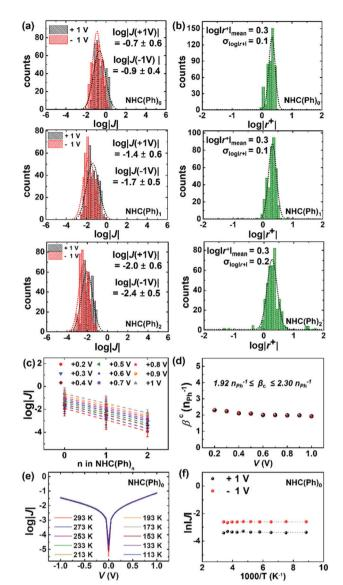
Fig. 2 Histograms of (a)  $\log |J|$  and (b)  $\log |r^+|$  at  $\pm 1.0$  V for NHC(Ph)<sub>n</sub> (n = 0, 1, and 2) SAM. (c) Linear correlation between the  $\log |J|$  and the molecular length. (d) Constant  $\beta^{c}$  value regardless of applied voltage. (e) Exemplary log|J|-V traces measured at low temperatures (from 113 to 293 K) for Au<sup>TS</sup>/NHC(Ph)<sub>0</sub>//Ga<sub>2</sub>O<sub>3</sub>/EGaIn junctions. (f) The corresponding Arrhenius plots.
