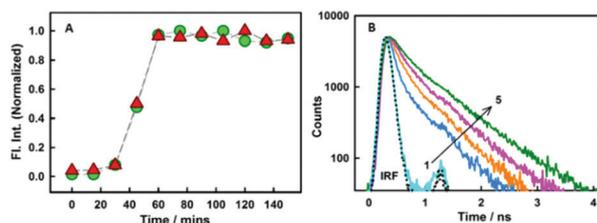
Fig. 3 (A) Normalized plot for the variation in intensity for styryl-11 (triangles) and thioflavin-T (circles). (B) Fluorescence decay traces for 10  $\mu\text{M}$  styryl-11 at various concentrations (in  $\mu\text{M}$ ) of insulin fibrils (1) 0 (2) 1.45 (3) 4.2 (4) 7 and (5) 19. The dotted line represents the instrument response function (IRF).
