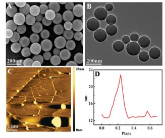
Fig. 3 (A) SEM image of SiO<sub>2</sub> microspheres; (B) TEM image of SiO<sub>2</sub> microspheres; (C) AFM image of SiO2-DNA hydrogel by HCR; and (D) height profile of SiO<sub>2</sub>-DNA hydrogel by HCR.
