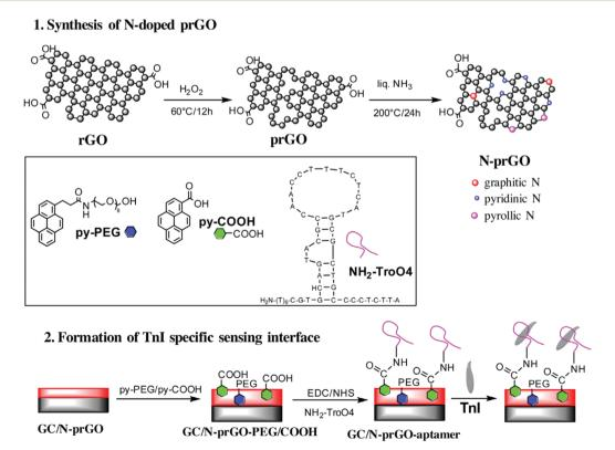
Fig. 11 Schematic illustration of the synthetic strategy for N-prGO and the preparation of an immunosensor for cTnl. Reproduced from ref. 144 with
