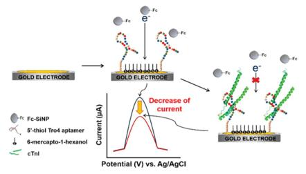
Fig. 1 Schematic illustration of voltammetric detection of cTnl. Upon immobilization of the cTnl aptamer on the surface of a gold working electrode, cTnI is added. The cTnI concentration was quantified by monitoring the decrease in SWV signal resulting from the hindered approaching of Fc-SiNPs. Reproduced from ref. 90 with permission.
