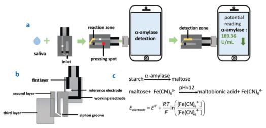
Fig. 8 (a) Schematic illustration of HSA detection using a smartphone-based sensor; (b) the three layers of the sensor; and (c) the reaction steps involved in HSA detection. Reproduced and adapted from ref. 124 with permission.
