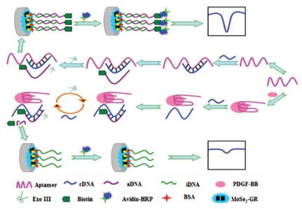
Fig. 6 Schematic illustration of aptasensor construction and the fundamentals of PGDF-BB detection using Exonuclease III-assisted signal amplification. Reproduced from ref. 117 with permission
